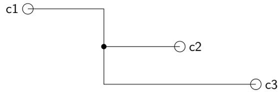
Figure 5: Splitting Connectors – Split Dot
