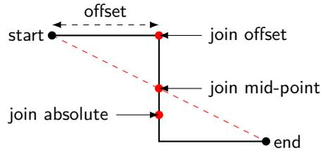
Figure 1: Stepped Simple Connector
