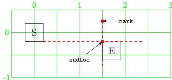
Figure 2: Straight Simple Connectors
